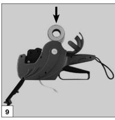
• Lay the roll securely into the appliance.
