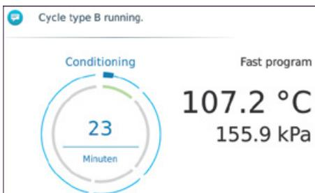
In the overpressure range steam is let off and regenerated, as a result of which the load is conditioned.
