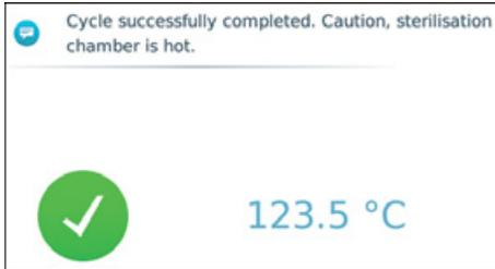
At the end of a program the pressure in the sterilisation chamber is matched to the ambient pressure.
