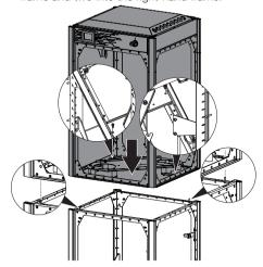
Push on and secure the noise insulation on the suction manifold of the compressor unit.
