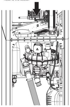
> Establish the compressed air connection for the compressor unit.
