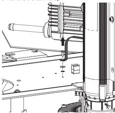
> Remove the clip for L bracket.
