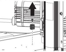
Mount the valve block with earth strap.
