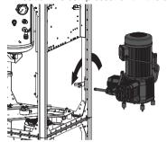
Mount the compressor unit on the retaining plate using four nuts. ΕN
